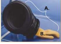
(30"). When the glove and sleeve are separated, the sleeve remains attached to the box. Glove sizes are interchangeable and almost any standard laboratory, surgical or disposable glove can be used. The glove and sleeve form a leak proof unit with O-ring construction integral with the box. The bellows allows cooling air circulation. Use with Scienceware® H50025-0320 Clamping Rings (see next page) to hold gloves in place. *Per pair.*
