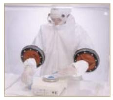
H50026). Fabricated of ten layers of silicone latex rubber, the 30 points of pliant material afford easy access and withdrawal while maintaining an excellent seal around the arm. Best for unconstrained use of delicate instruments inside the Glove Box where operations with gloves can be awkward. *Per pair.*
